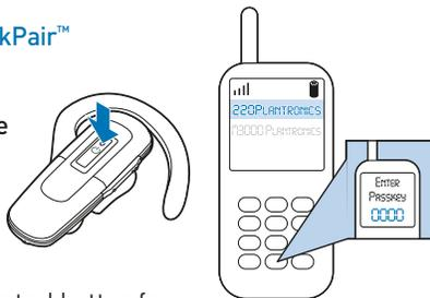
**Step 2:** Use your device's menu to enter its pairing mode and select **220Plantronics** on the display. **0000** is the pairing passkey.
