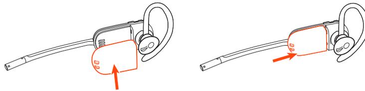
**NOTE** This product has a replaceable battery. Only use the battery type supplied by Plantronics.
