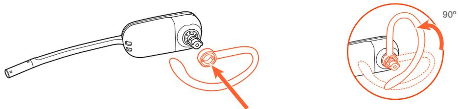
**NOTE** Ensure the ear loop is flat against the headset before rotating.
