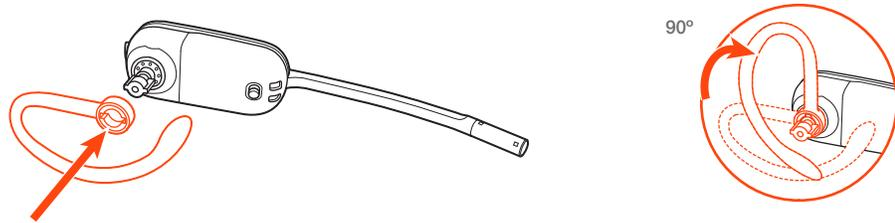
**NOTE** Ensure the ear loop is flat against the headset before rotating.
