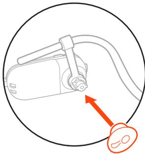
**NOTE** Ensure the large end of the ear tip points to the microphone.
