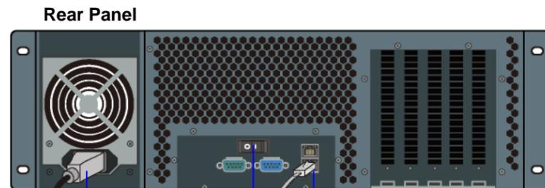
Power Cable Off/On Switch LAN1 Connection
