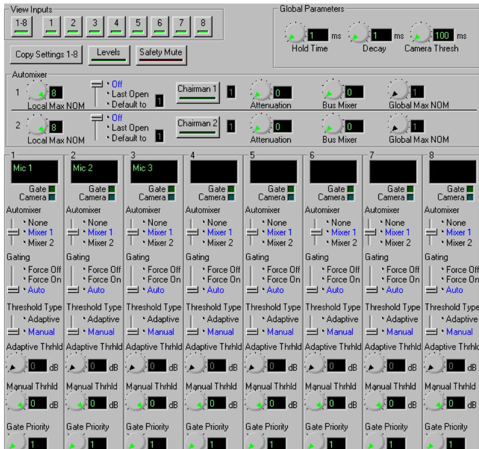
Figure 10. Automixer controls on the Automixer Page.
