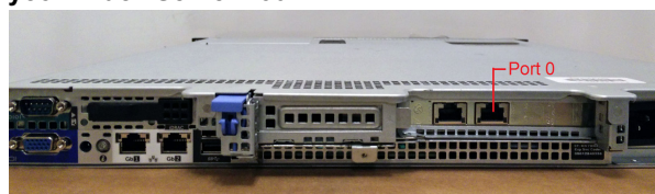
Figure 2: Port 0 Location for Polycom Rack Server 230
