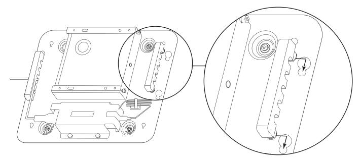
10 Attach the cover to the wall plate by inserting the four bolts into the top of the four corner keyhole slots and sliding them down to lock in place.
