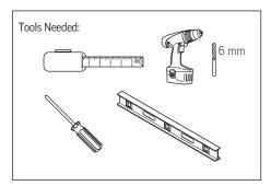
Drill four 6 mm holes in the wall, 200 mm apart, to a depth of 40 mm.
