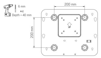
3 Attach the four mounting screws using the outer M4 riveting studs.
