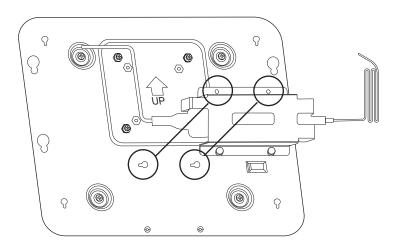
Slide the PC into the PC holder and attach two thumb screws.
