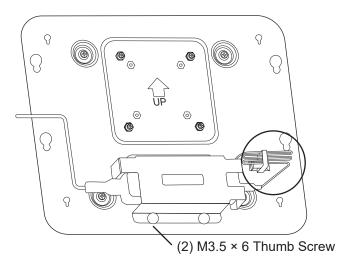
8 Attach the PC to the plate by sliding the PC holder keyholes onto the four mounting screws.
