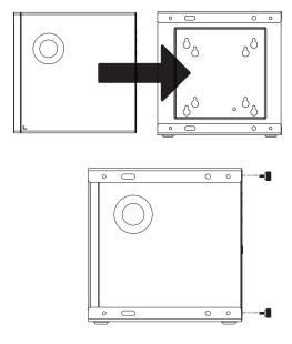
6 Attach two thumb screws at the bottom of the PSU holder. Wrap the cable wrap around the power cable.
