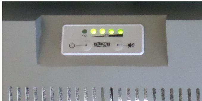
2. It is best to **leave the cart plugged into a wall outlet** whenever the unit is parked for a while, or longer. The cart's charger is automatic and will not overcharge the battery, but will maintain an optimum high state of charge.
