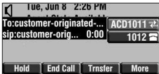
**Figure 27: Customer-Originated Trace Screen on a VVX 600 Phone**
