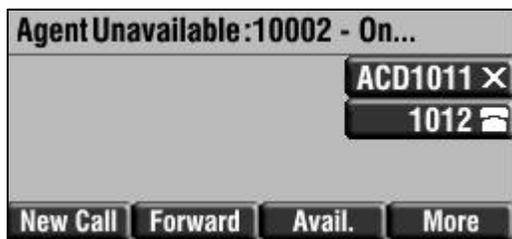
**Figure 21: VVX 600 Phone's Main Screen with Unavailable Reason Code Displayed**
