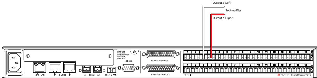
Figure 4. SoundStructure connections to an external stereo amplifier.
