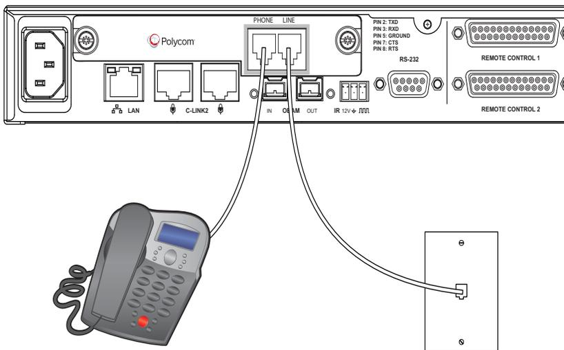
When the SoundStructure TEL1 device takes its *LINE* interface off-hook by using the SoundStructure API (See the SoundStructure Command Reference manual) `phone_connect` command, the audio from the telephone *LINE* interface is routed through the SoundStructure TEL1 and into the SoundStructure for audio processing. When off-hook, the TEL1 seizes the line from the handset and will not release it to the handset until the TEL1 is placed back on-hook (in other words, hung-up).
